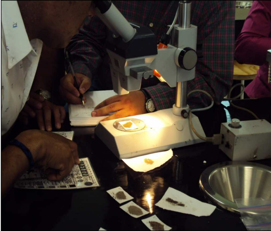
Figure. 2. Practice in the lab with stereo microscopy, Munsell chart, the geotechnical gauge and table from Powers and Krumbein
